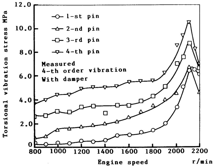
Fig. 11 Amplitude curves of torsional vibration stress at crank pin center (with damper, 4-th order vibration, measured)
