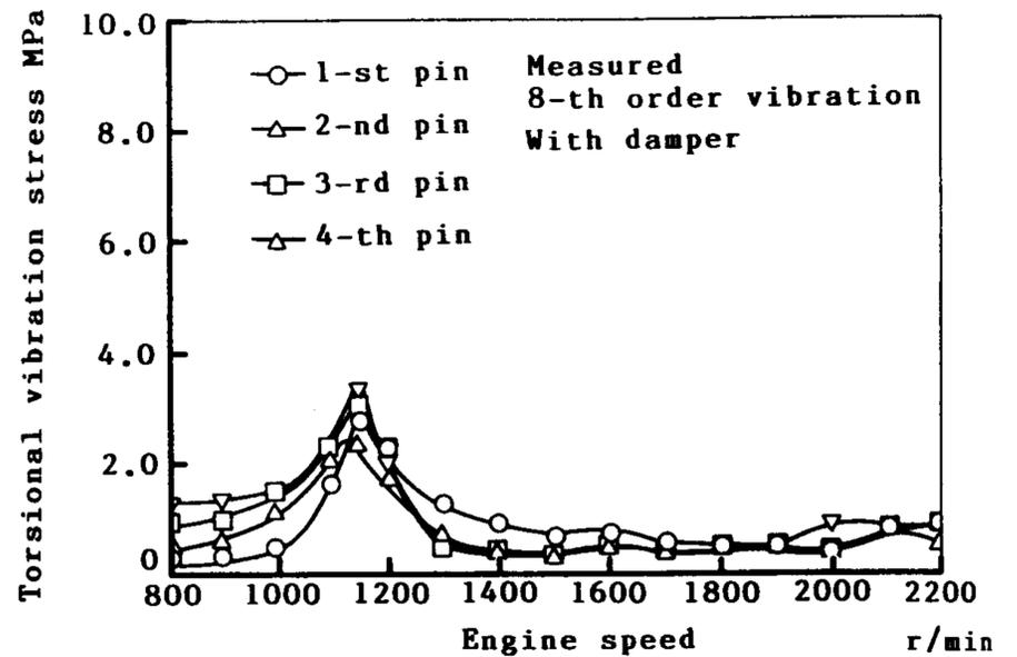
Fig. 12 Amplitude curves of torsional vibration stress at crank pin center (with damper, 8-th order vibration, measured)
