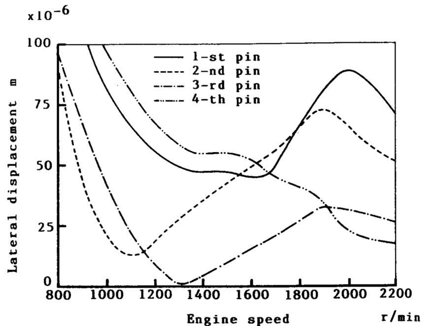
Fig. 24 Amplitude curves of lateral displacement at crank pin center (with damper, 4-th order vibration, computed)
