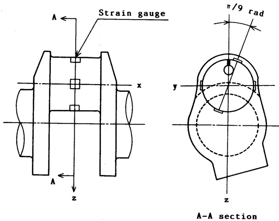
Fig. 8 Adhesived location of strain gauge at crank pin center
