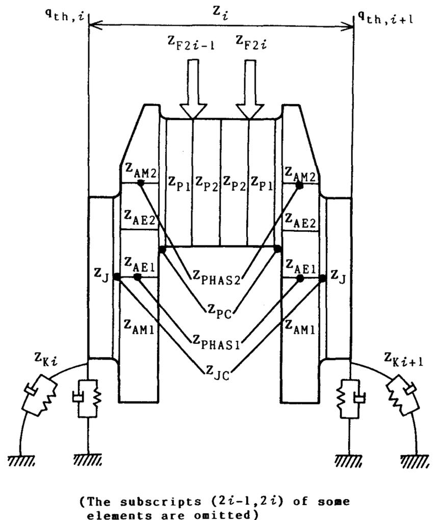
Fig. 6 Detailed vibration model of *i*-th crank throw for transfer matrix method
