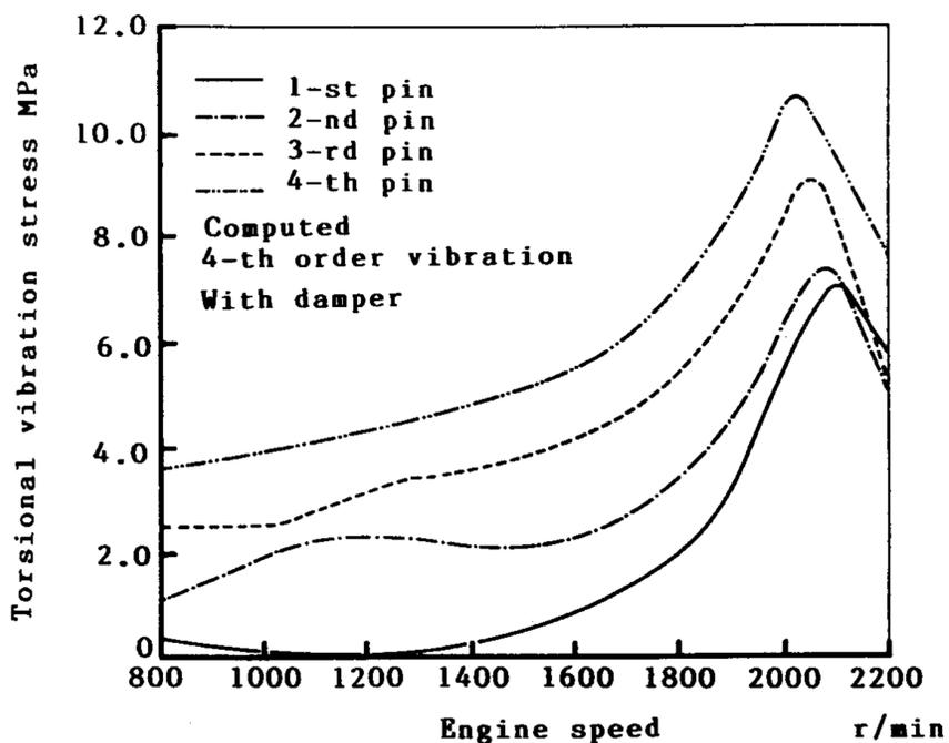
Fig. 13 Amplitude curves of torsional vibration stress at crank pin center (with damper, 4-th order vibration, computed)
