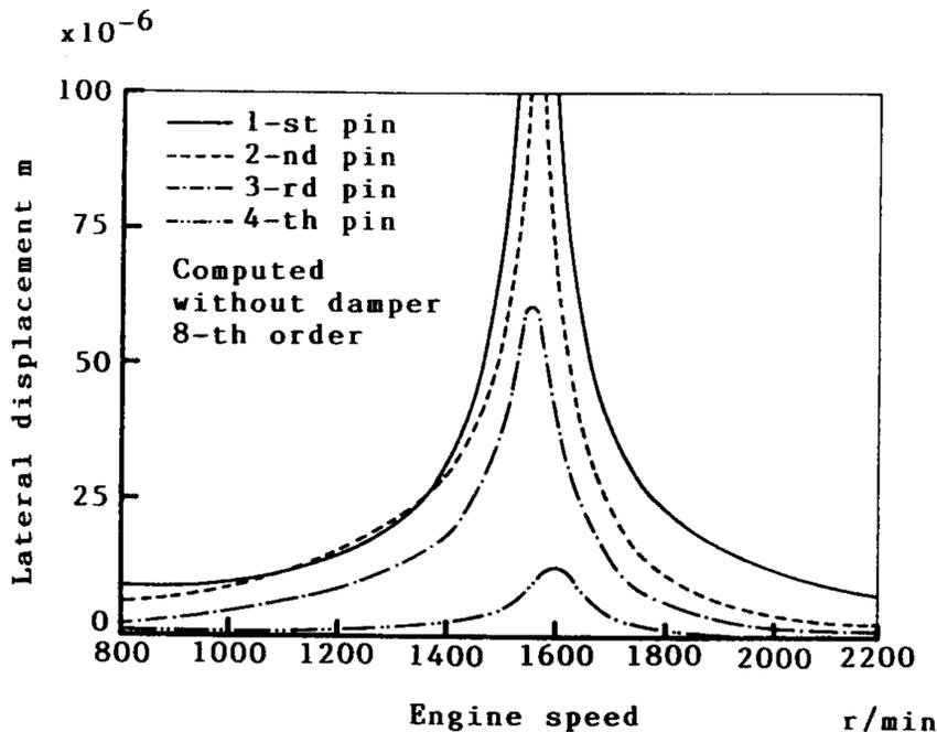
Fig. 25 Amplitude curves of lateral displacement at crank pin center (without damper, 8-th order vibration, computed)
