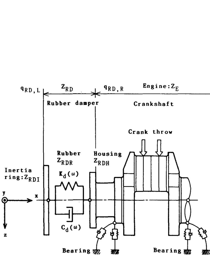
Fig. 5 Vibration model of crankshaft with a rubber damper for transfer matrix method
