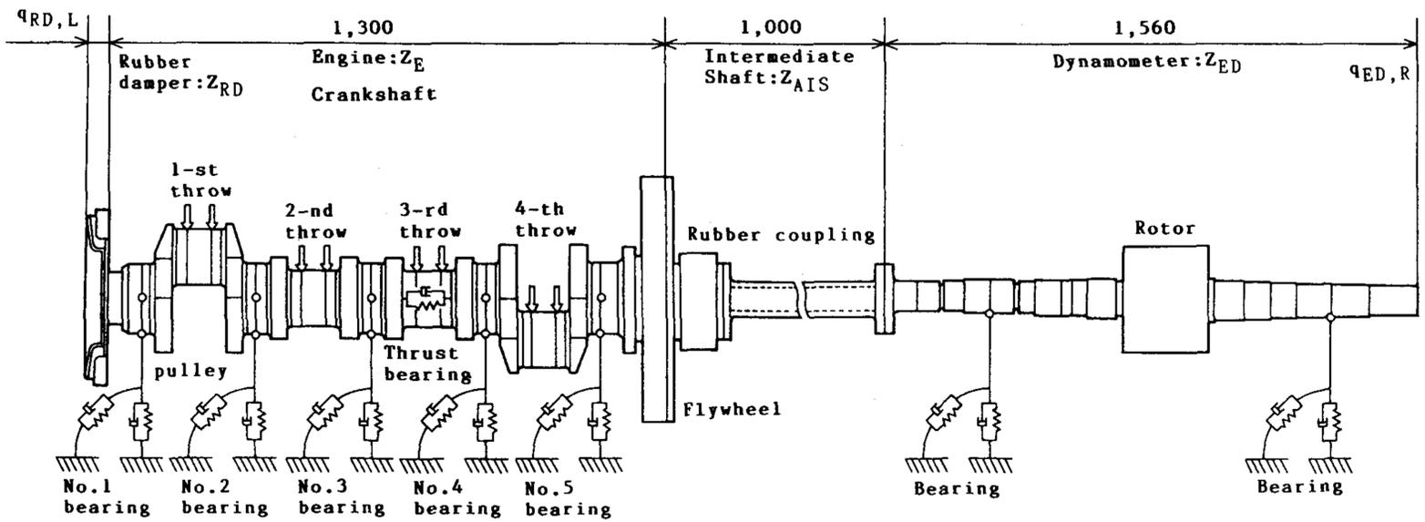
Fig. 4 Whole vibration model of a Vee 8-cylinder engine crankshaft for transfer matrix method
