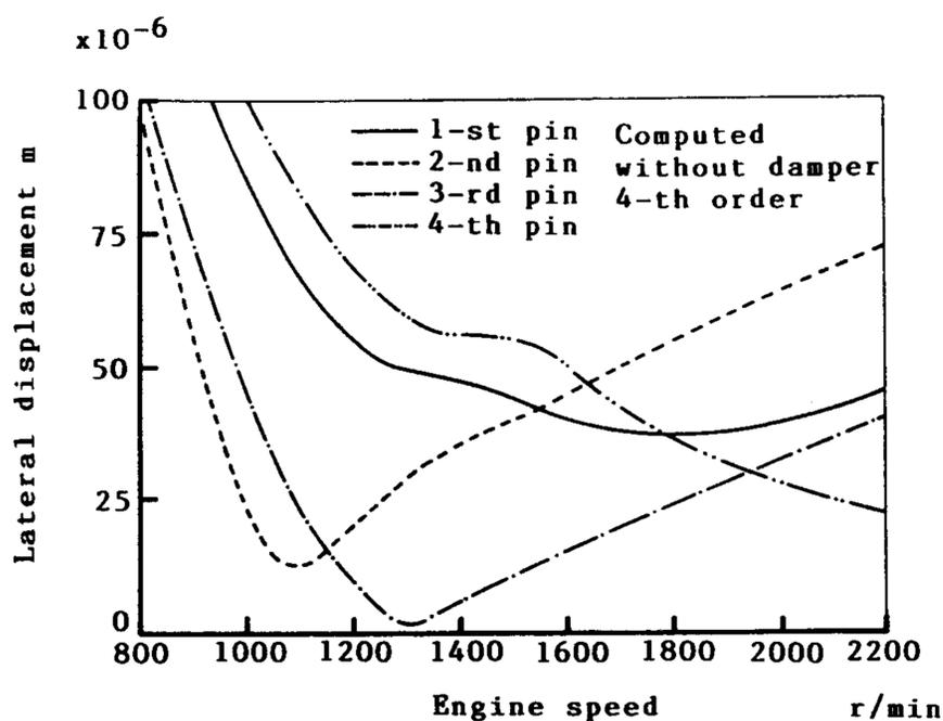
Fig. 23 Amplitude curves of lateral displacement at crank pin center (without damper, 4-th order vibration, computed)
