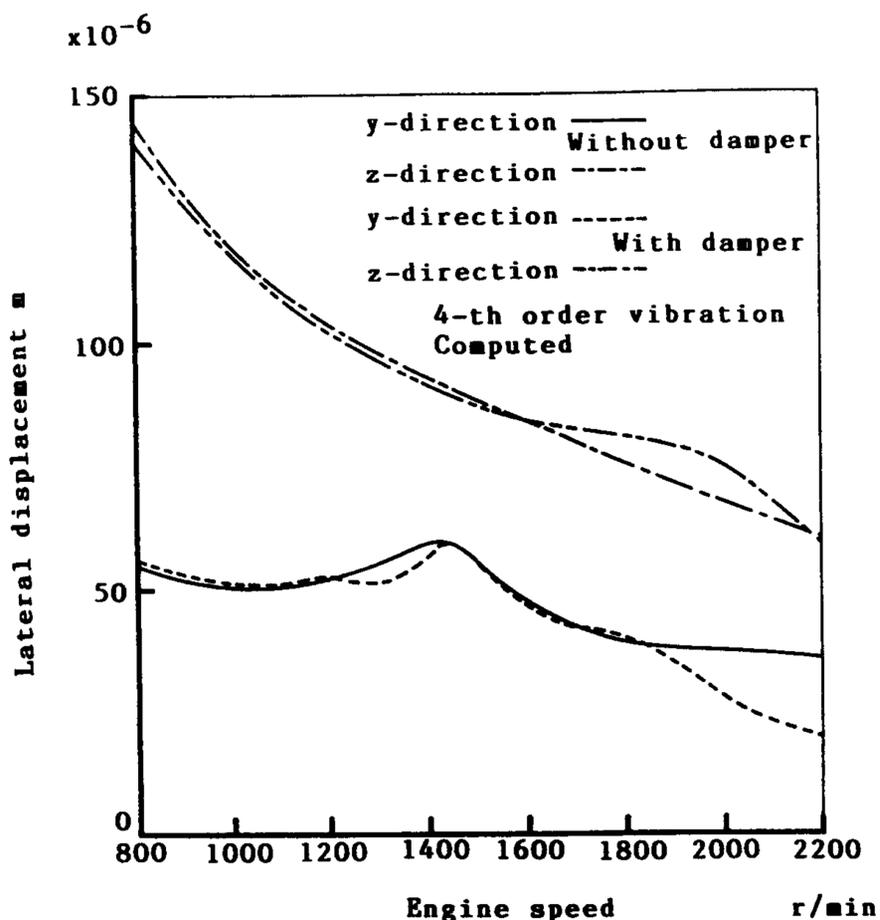
Fig. 21 Amplitude curves of lateral displacement at pulley end (4-th order vibration, computed)
