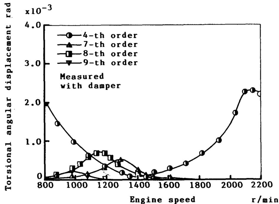
Fig. 9 Amplitude curves of torsional angular displacement at pulley end (with damper, measured)
