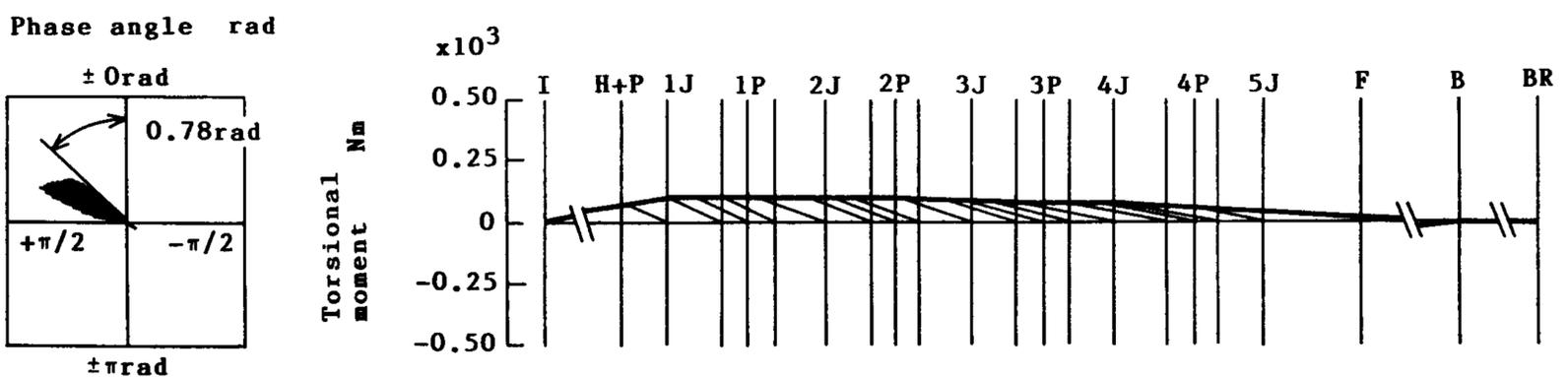
Fig. 20 Vibration mode of torsional moment (with damper, 8-th order vibration, resonant engine speed 1,039 r/min)
