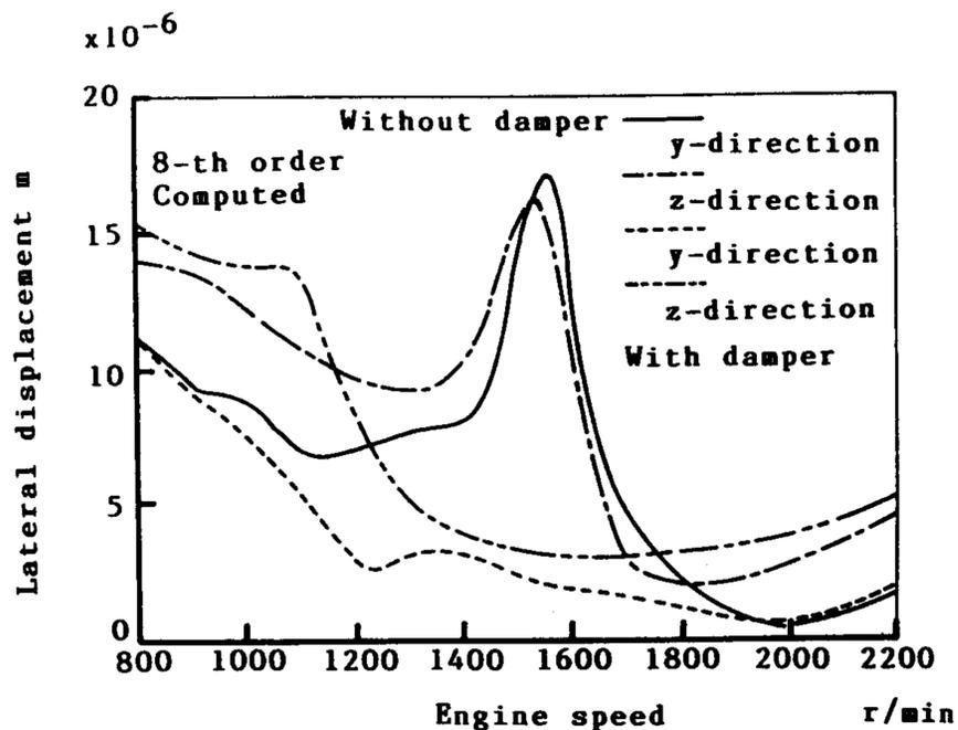
Fig. 22 Amplitude curves of lateral displacement at pulley end (8-th order vibration, computed)
