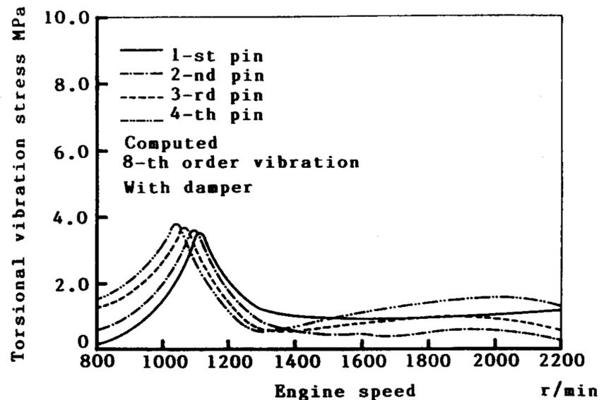
Fig. 14 Amplitude curves of torsional vibration stress at crank pin center (with damper, 8-th order vibration, computed)
