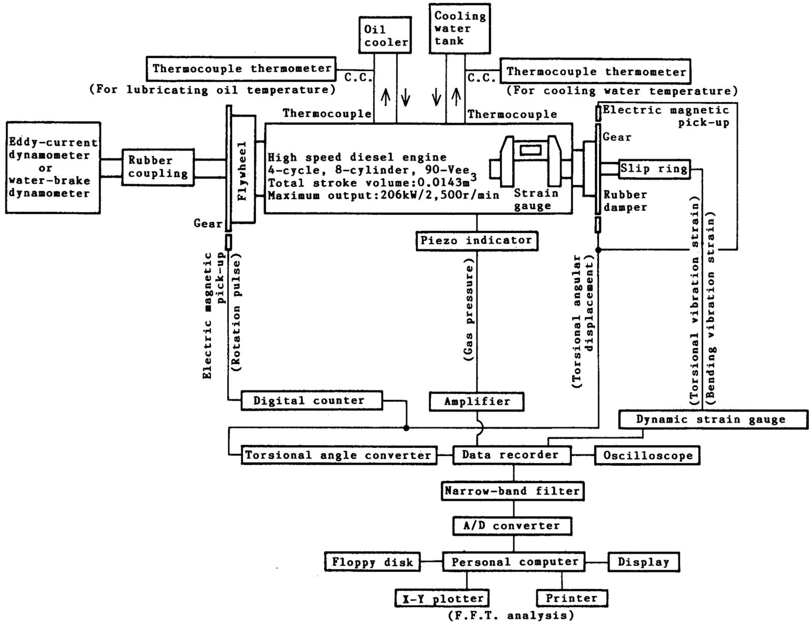
Fig. 7 Schematic diagram for vibration measurement of crankshaft system
