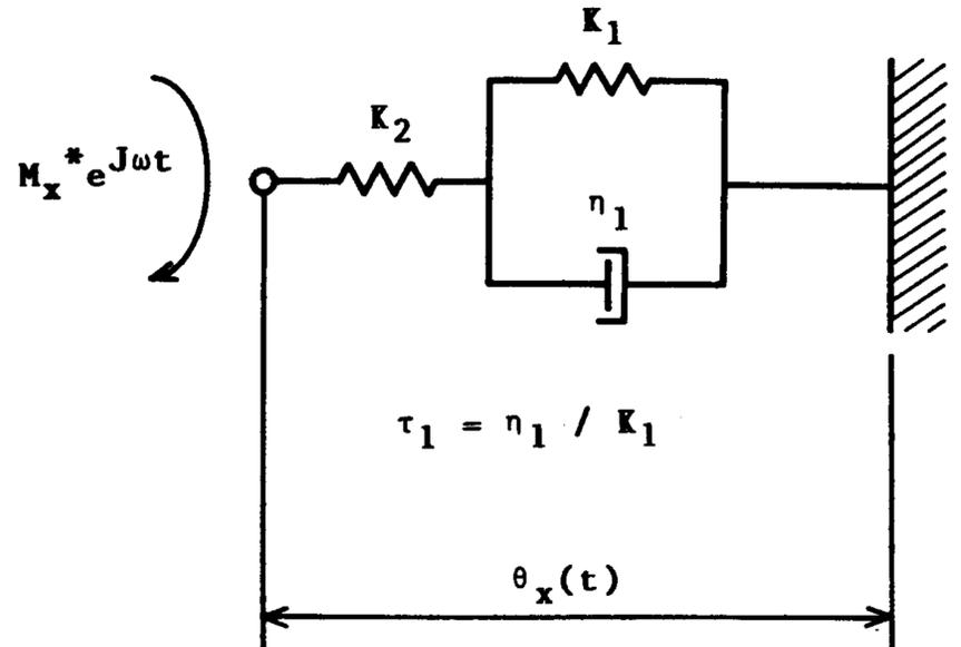
Fig. 2 Three-element Maxwell model
