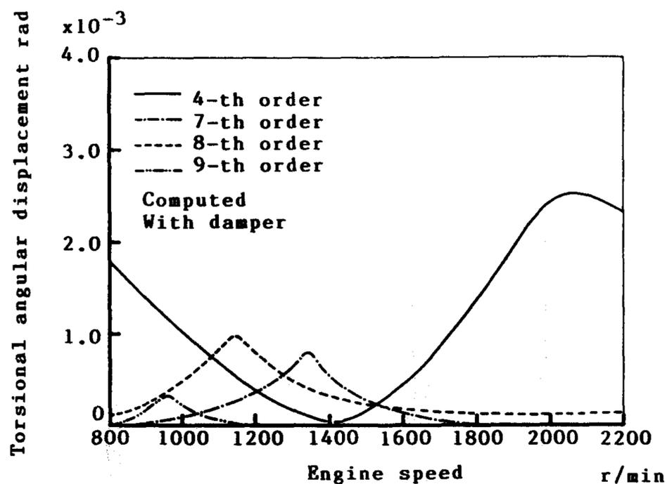
Fig. 10 Amplitude curves of torsional angular displacement at pulley end (with damper, computed)
