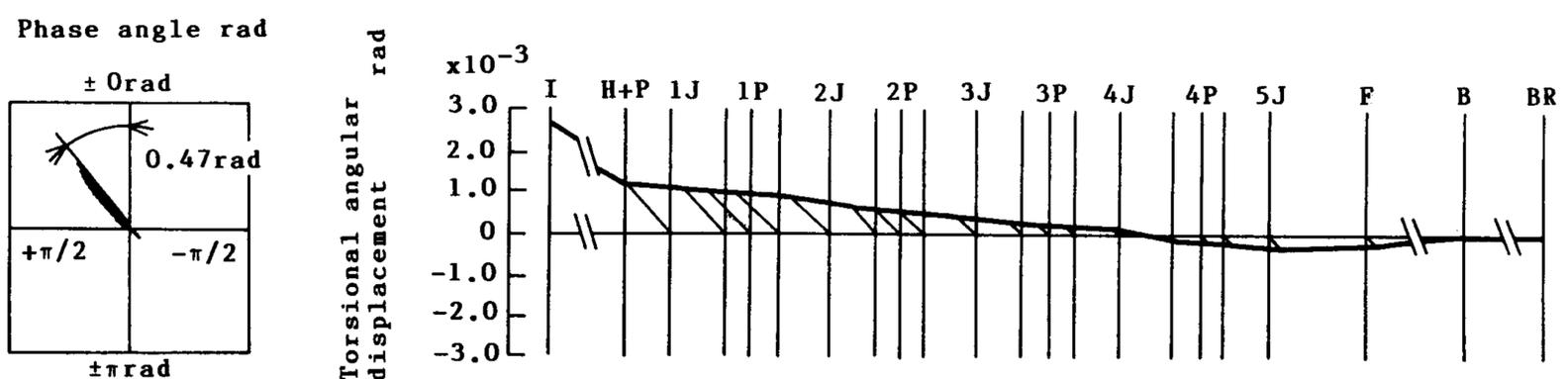
**Fig. 16** Vibration mode of torsional angular displacement (with damper, 4-th order vibration, resonant engine speed 2,110 r/min)
