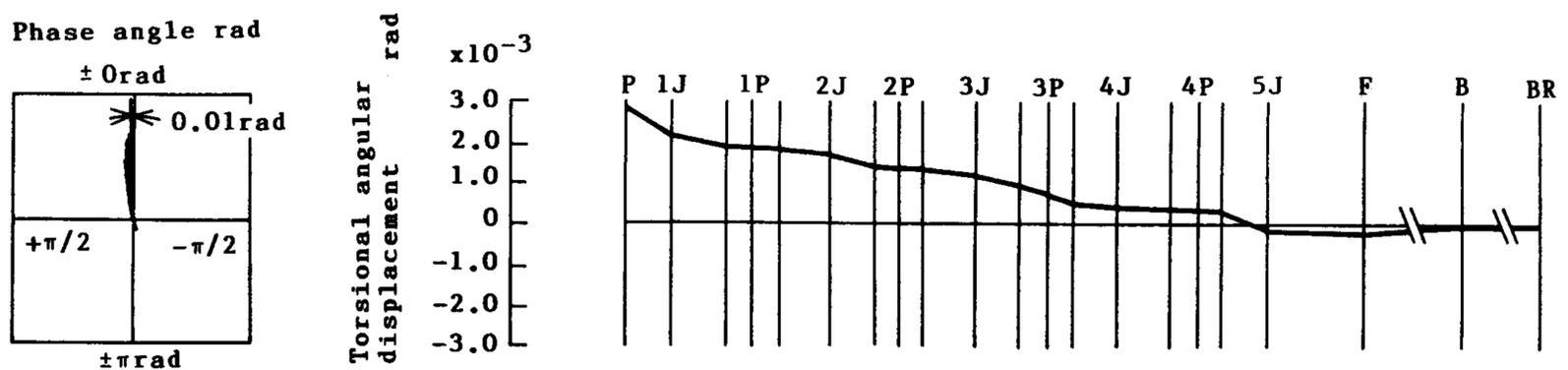
**Fig. 15** Vibration mode of torsional angular displacement (without damper, 8-th order vibration, resonant engine speed 1,580 r/min)
