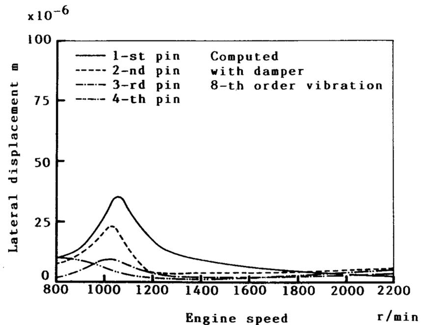
Fig. 26 Amplitude curves of lateral displacement at crank pin center (with damper, 8-th order vibration, computed)
