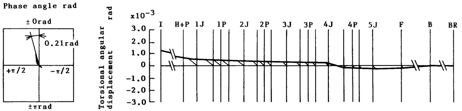
Fig. 17 Vibration mode of torsional angular displacement (with damper, 8-th order vibration, resonant engine speed 1,100 r/min)
