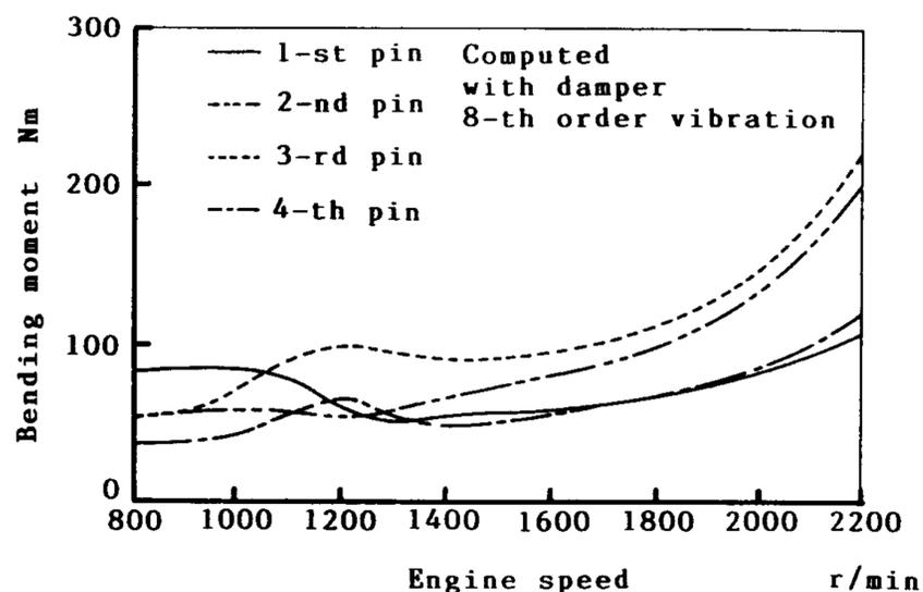
Fig. 27 Amplitude curves of bending moment at crank pin center (with damper, 8-th order vibration, computed)
