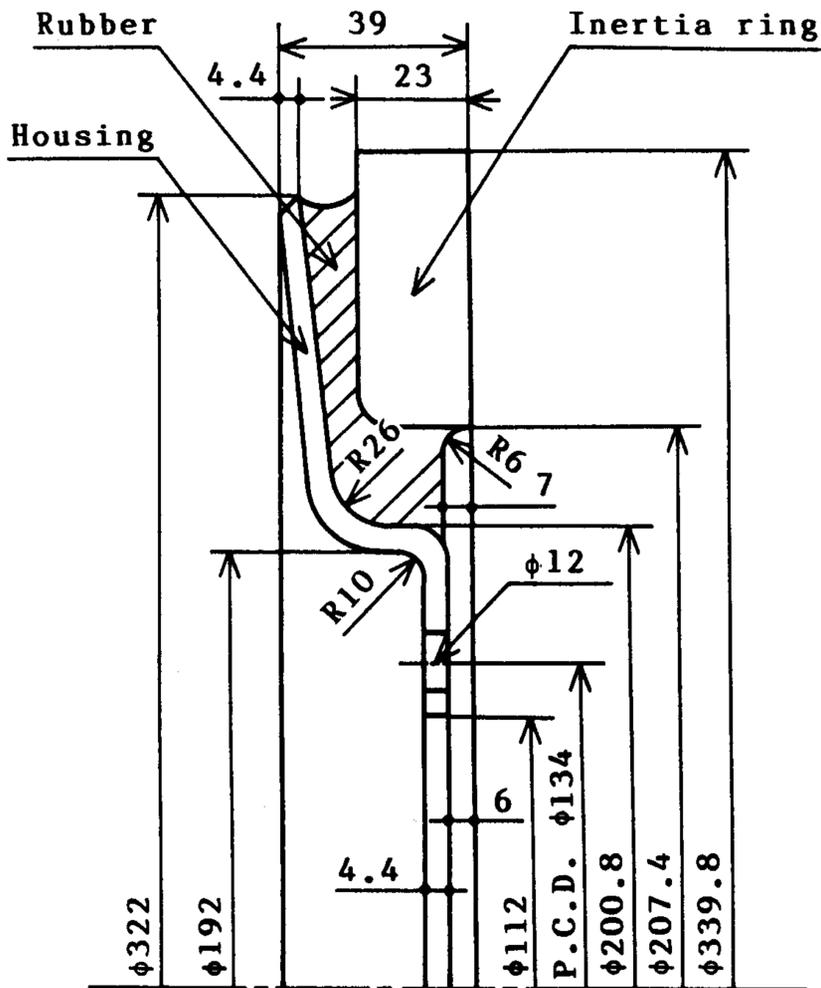
Fig. 1 Shape and dimensions of test rubber damper
