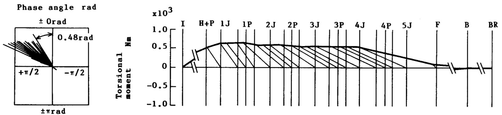
Fig. 19 Vibration mode of torsional moment (with damper, 4-th order vibration, resonant engine speed 2,020 r/min)
