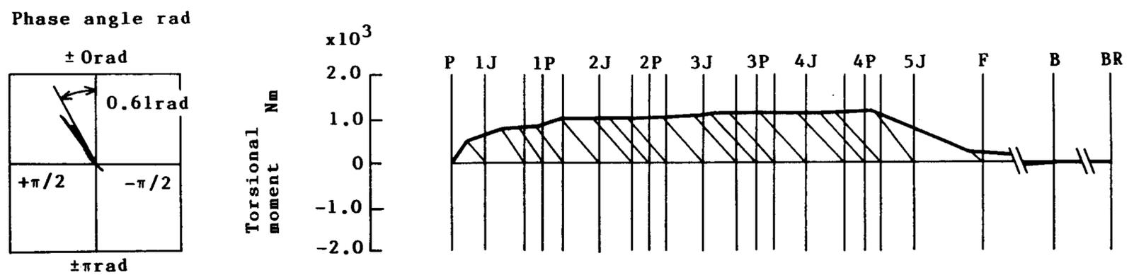
Fig. 18 Vibration mode of torsional moment (without damper, 8-th order vibration, resonant engine speed 1,523 r/min)
