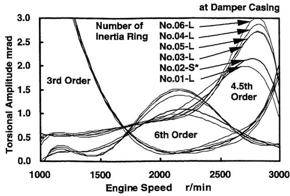
Fig. 6(a) Torsional Amplitude Curves of Damper Casing on Conditions of Lateral Gap Changes (Peripheral Gap: Constant, Kinematic Viscosity:  $0.05 \text{ m}^2/\text{s}$ )
