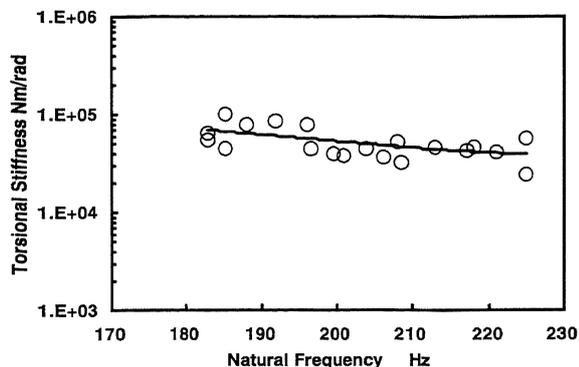
Fig. 11(a) Relationship between Torsional Stiffness and Natural Frequency (Kinematic Viscosity:  $0.30 \text{ m}^2/\text{s}$ )
