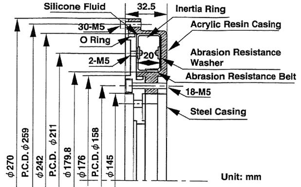
**Fig. 1** Geometry of Viscous-Fluid Damper**Table 2(a)** Dimensions of Damper Inertia Ring (Change of Lateral Gap)
