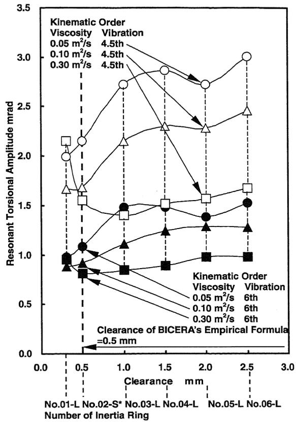
Fig. 9(a) Relationship between Resonant Torsional Amplitude and Clearance Gap (Gap Change of Only Lateral Clearance)
