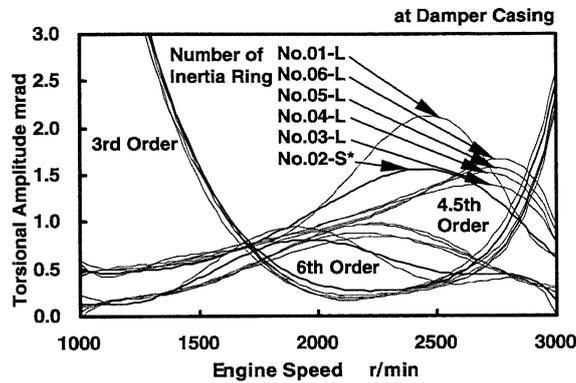
Fig. 6(c) Torsional Amplitude Curves of Damper Casing on Conditions of Lateral Gap Changes (Peripheral Gap: Constant, Kinematic Viscosity:  $0.30 \text{ m}^2/\text{s}$ )
