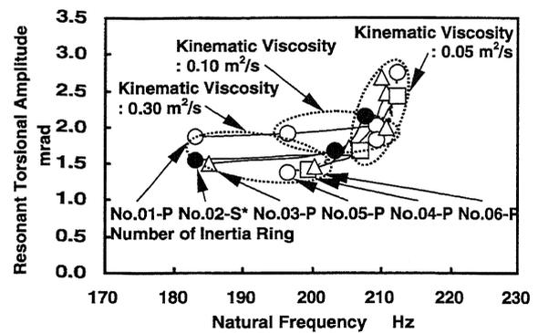
Fig. 7(b) Relationship between Resonant Torsional Amplitude and Natural Frequency by Change of Kinematic Viscosity (Peripheral Gap: Change, Lateral Gap: Constant, 4.5th Order Vibration)
