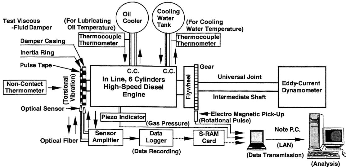
Fig. 2 Schematic Diagram of Simultaneously Measuring System of Torsional Vibration Waveforms at Two Points
