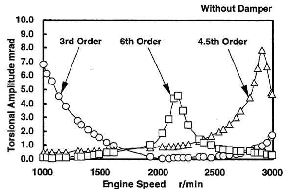
Fig. 3 Amplitude Curves of Torsional Angular Displacements at Pulley End (Without Damper)
