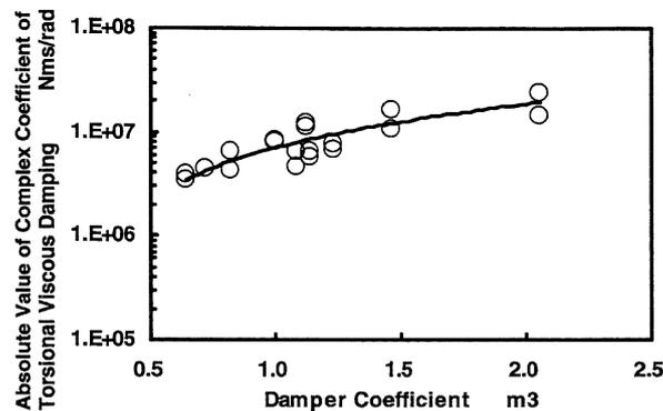
Fig. 12(c) Relationship between Absolute Value of Complex Coefficient of Torsional Viscous Damping and Damper Coefficient (Kinematic Viscosity:  $0.30 \text{ m}^2/\text{s}$ )
