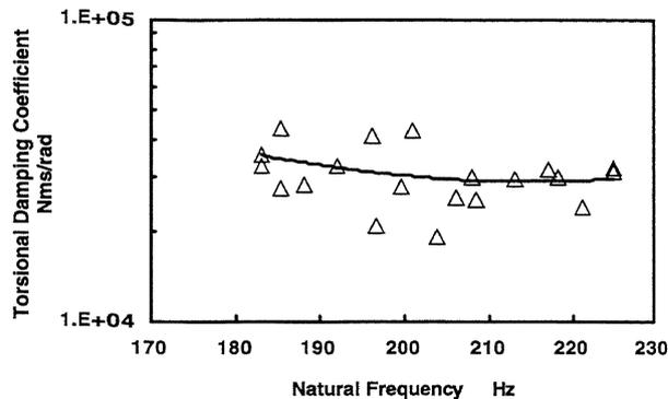
Fig. 11(b) Relationship between Torsional Damping Coefficient and Natural Frequency (Kinematic Viscosity:  $0.30 \text{ m}^2/\text{s}$ )
