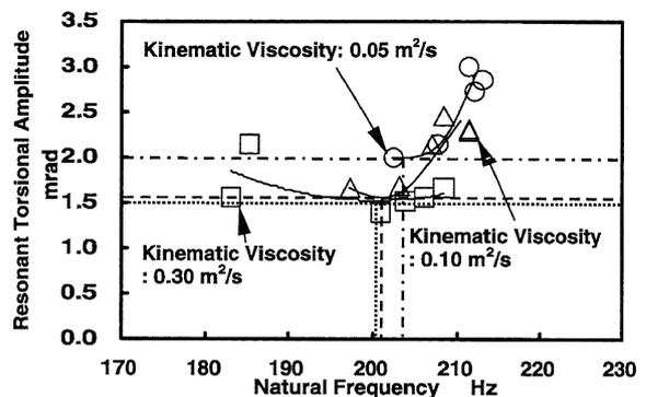
Fig. 8(b) Relationship between Resonant Torsional Amplitude and Natural Frequency by Gap Change of Clearance in Every Kinematic Viscosity (Lateral Gap: Change, Peripheral Gap: Constant, 4.5th Order Vibration)
