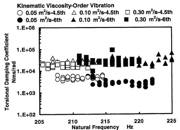
Fig. 10(b) Relationship between Torsional Damping Coefficient and Natural Frequency (Number of Inertia Ring: No. 04-P)
