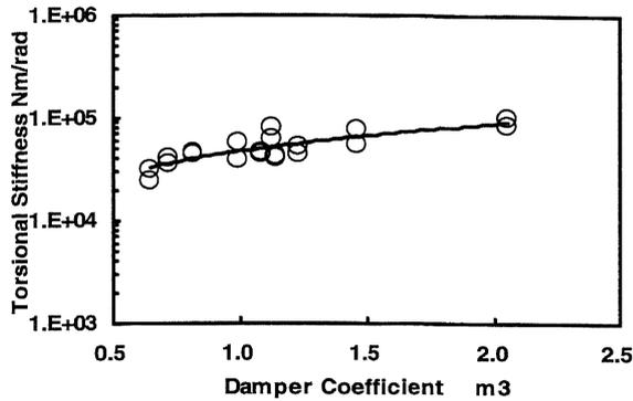
Fig. 12(a) Relationship between Torsional Stiffness and Damper Coefficient (Kinematic Viscosity:  $0.30 \text{ m}^2/\text{s}$ )
