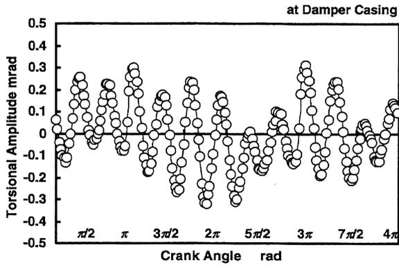
Fig. 4(a) Waveform of Torsional Angular Displacement at Damper Casing (Inertia Ring No. 02-S\*, 6th Order Resonant Engine Speed: 2170 r/min)
