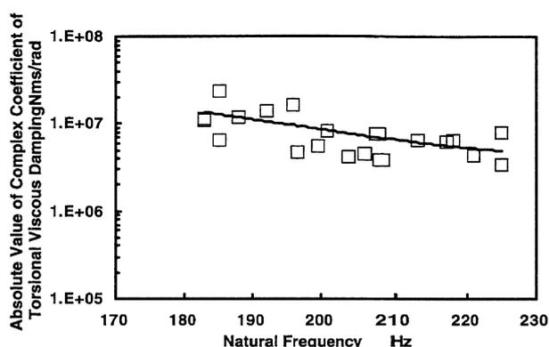
Fig. 11(c) Relationship between Absolute Value of Complex Coefficient of Torsional Viscous Damping and Natural Frequency (Kinematic Viscosity:  $0.30 \text{ m}^2/\text{s}$ )
