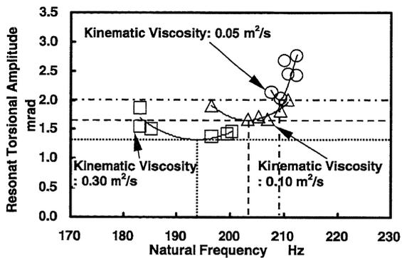
Fig. 8(a) Relationship between Resonant Torsional Amplitude and Natural Frequency by Gap Change of Clearance in Every Kinematic Viscosity (Peripheral Gap: Change, Lateral Gap: Constant, 4.5th Order Vibration)
