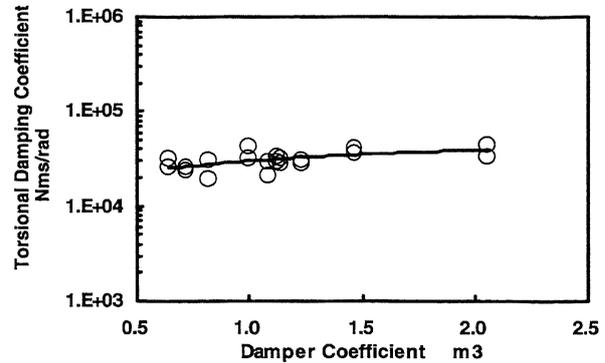
Fig. 12(b) Relationship between Torsional Damping Coefficient and Damper Coefficient (Kinematic Viscosity:  $0.30 \text{ m}^2/\text{s}$ )
