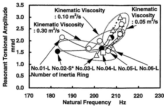
Fig. 7(a) Relationship between Resonant Torsional Amplitude and Natural Frequency by Change of Kinematic Viscosity (Lateral Gap: Constant, Peripheral Gap: Constant, 4.5th Order Vibration)
