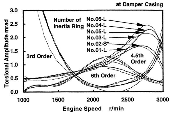
Fig. 6(b) Torsional Amplitude Curves of Damper Casing on Conditions of Lateral Gap Changes (Peripheral Gap: Constant, Kinematic Viscosity:  $0.10 \text{ m}^2/\text{s}$ )
