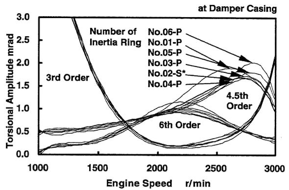
Fig. 5(b) Torsional Amplitude Curves of Damper Casing on Conditions of Peripheral Gap Changes (Lateral Gap: Constant, Kinematic Viscosity: 0.10 m<sup>2</sup>/s)
