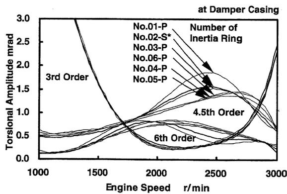
Fig. 5(c) Torsional Amplitude Curves of Damper Casing on Conditions of Peripheral Gap Changes (Lateral Gap: Constant, Kinematic Viscosity: 0.30 m<sup>2</sup>/s)
