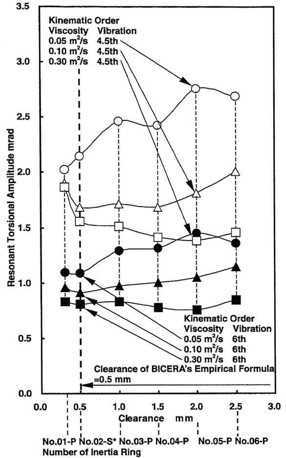
Fig. 9(b) Relationship between Resonant Torsional Amplitude and Clearance Gap (Gap Change of Only Peripheral Clearance)
