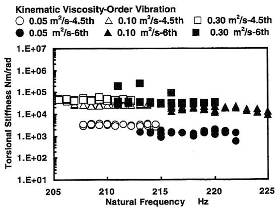
Fig. 10(a) Relationship between Torsional Stiffness and Natural Frequency (Number of Inertia Ring: No. 04-P)
