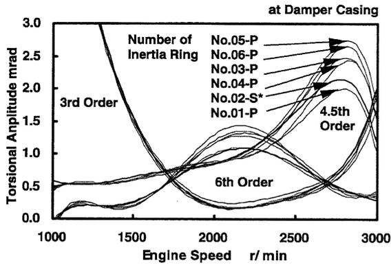
Fig. 5(a) Torsional Amplitude Curves of Damper Casing on Conditions of Peripheral Gap Changes (Lateral Gap: Constant, Kinematic Viscosity: 0.05 m<sup>2</sup>/s)
