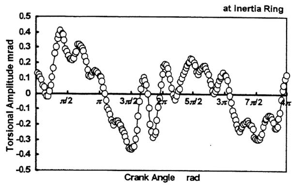
Fig. 4(b) Waveform of Torsional Angular Displacement at Damper Inertia Ring (Inertia Ring No. 02-S\*, 6th Order Resonant Engine Speed: 2170 r/min)
