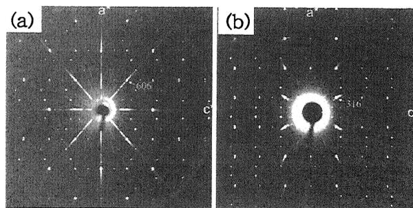
Fig. 3 Zero layer (a) and first layer (b) X-ray precession photographs of the  $\text{ErRh}_3\text{B}_2$  crystal in [010] zone axis.
