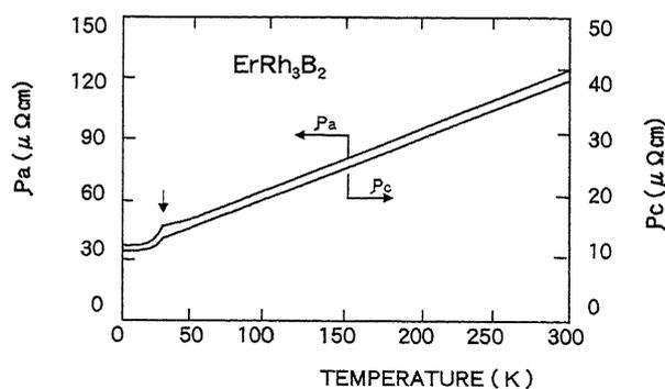
Fig. 5 Temperature dependence of the electric resistivity parallel and perpendicular to the  $c$ -axis of  $\text{ErRh}_3\text{B}_2$ .
