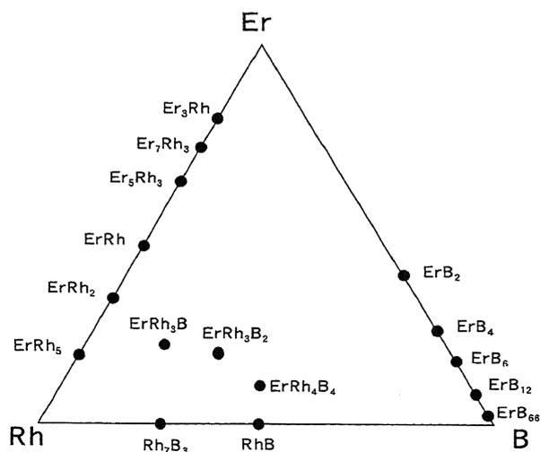
Fig. 1 Tentative phase diagram in the system of Er-Rh-B.
