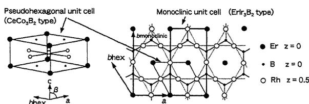
Fig. 4 Crystal structure of  $RT_3\text{B}_2$  ( $R$ =rare earth element,  $T$ =transition metal) compounds showing the relationship between the hexagonal  $\text{CeCo}_3\text{B}_2$  type structure and the monoclinic  $\text{ErIr}_3\text{B}_2$  type structure.
