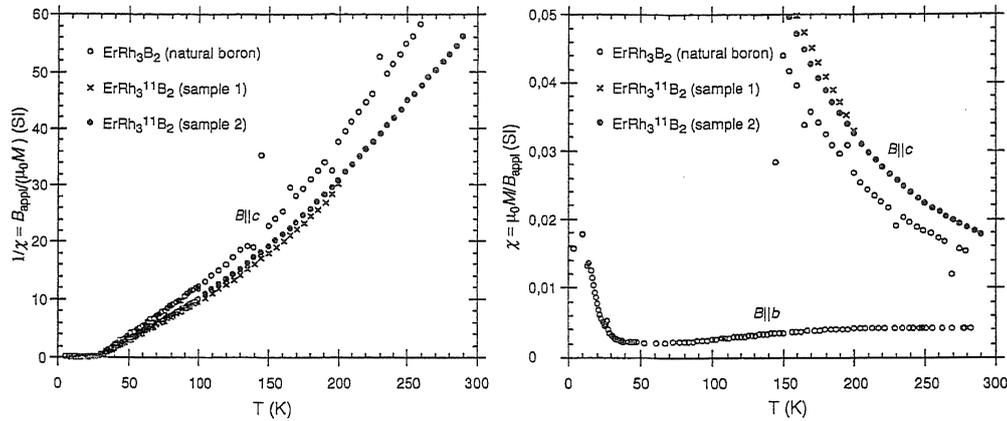
Fig. 6 Magnetic data for parallel and perpendicular to the  $c$ -axis of  $\text{ErRh}_3\text{B}_2$ . The inverse susceptibility  $1/\chi = B_{\text{app}}/\mu_0 M$  is shown on the left and the susceptibility  $\chi = \mu_0 M/B_{\text{app}}$  in low magnetic field on the right.
