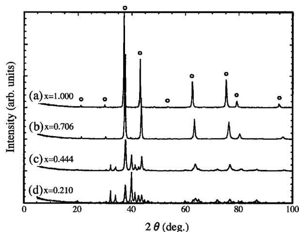
Fig. 2 XRD profiles for  $\text{GdRh}_3\text{B}_x$  with  $x = 1.000$  (a),  $x = 0.706$  (b),  $x = 0.444$  (c) and  $x = 0.210$  (d).
