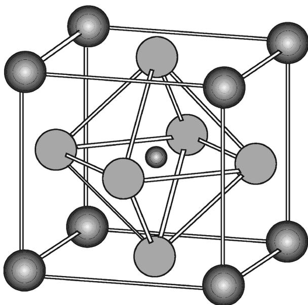
Fig. 1 Arrangement of atoms in the perovskite-type  $\text{GdRh}_3\text{B}$ . Large black, large gray and small black circles represent Gd, Rh and B atoms, respectively.
