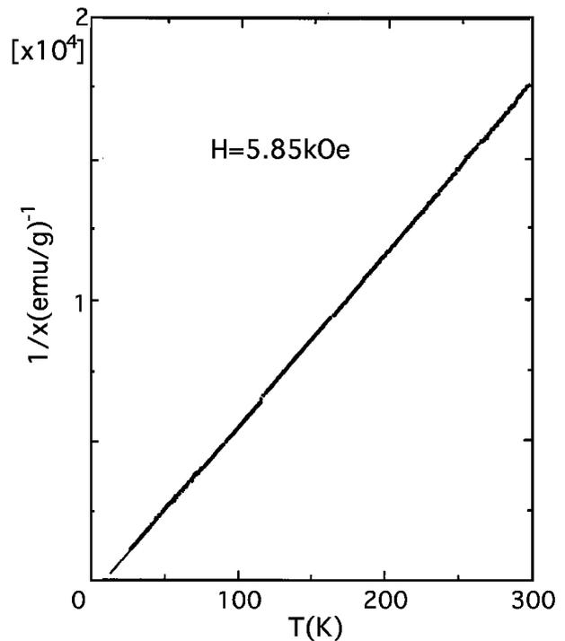
Fig. 6 Inverse magnetic susceptibility vs temperature  $T$  for  $\text{GdRh}_3\text{B}$ . ( $H = 5.85$  kOe)
