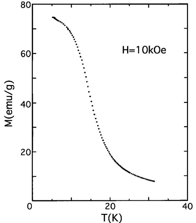
Fig. 5 Magnetization vs temperature  $T$  for  $\text{GdRh}_3\text{B}$ . ( $H = 10$  kOe)
