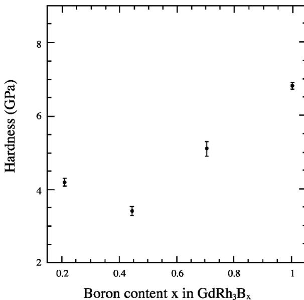
Fig. 4 Vickers microhardness for  $\text{GdRh}_3\text{B}_x$  as a function of the boron content,  $x$ .
