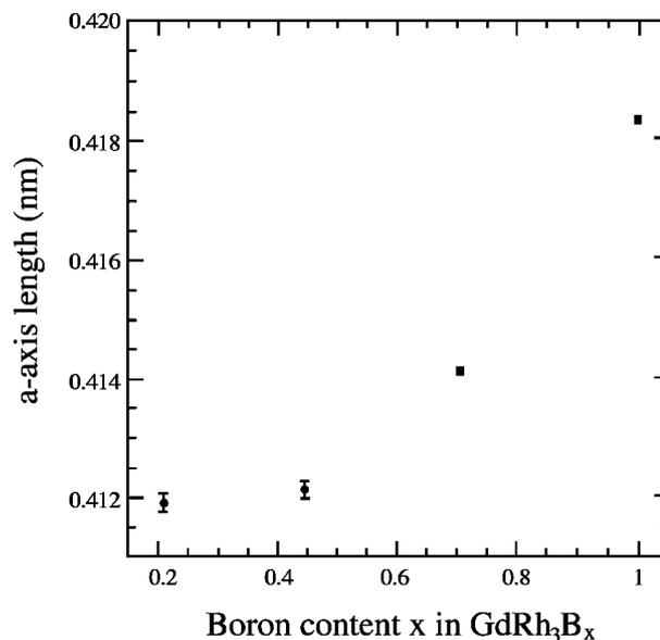
Fig. 3 The variation of lattice constant  $a$  as a function of boron concentration  $x$  in  $\text{GdRh}_3\text{B}_x$ .
