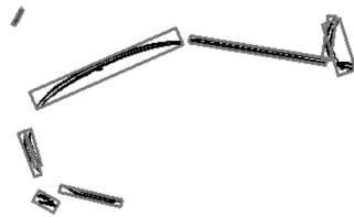
Fig. 13 Rectangles enveloping chip edge images.
