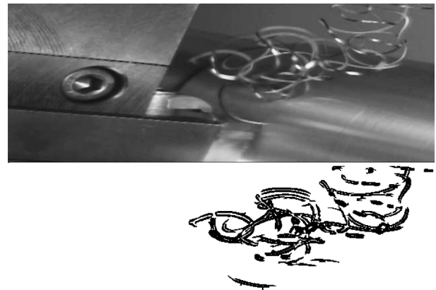
Fig. 11 Chip tangled in medium density.
