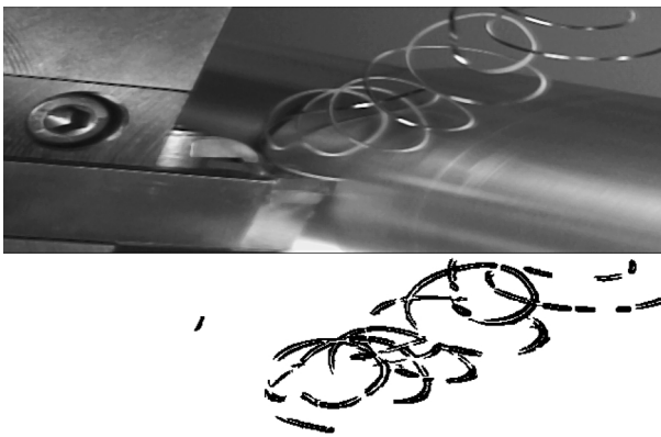
Fig. 10 Chip tangled in low density.
