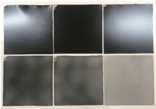
Fig.10 Painted with volcanic ash and powder paint From the top left, the volcanic ash contamination rate is 1x, 3x, 5x, 15x, and 30x. The lower right is a blank sample.
