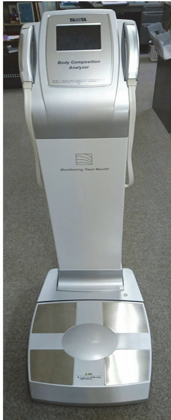
Fig.4. 8-electrode segmental bioelectrical impedance analysis (MC-190, TANITA) .
