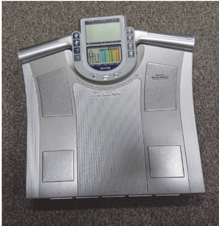
Fig.8. 8-electrode segmental bioelectrical impedance analysis (BC-621, TANITA) .
