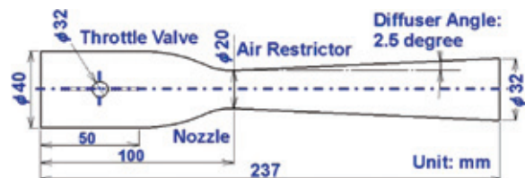
Figure 9 Dimension of Air Restrictor (Three-Dimensional Solid CAD Model) [Shape 02, Diffuser Angle: 2.5 [degree]]
