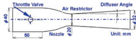
Figure 6 Basic CFD Model (Three-Dimensional Solid CAD Model) [Shape.] of Air Restrictor for SFJ Vehicle
