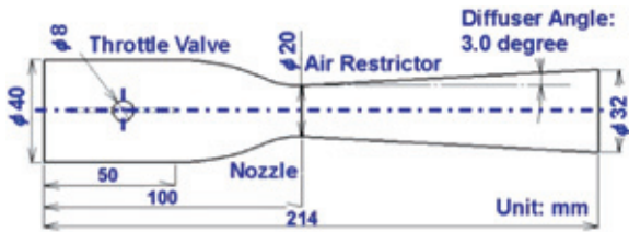
Figure 11 Dimension of Air Restrictor (Three-Dimensional Solid CAD Model) [Shape 03, Diffuser Angle: 3.0 [degree]]
