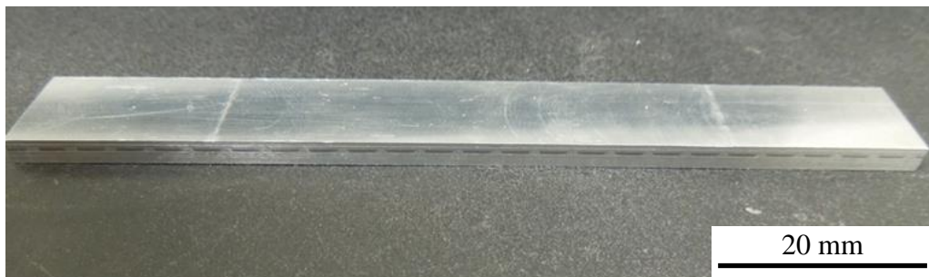
Fig. 4.13 Developed superplastic vibration-damping steel sheet composite
