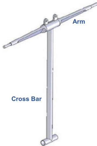
Figure 4 Three-Dimensional Solid CAD Model of Rear Stabilizer for Rear Suspension
