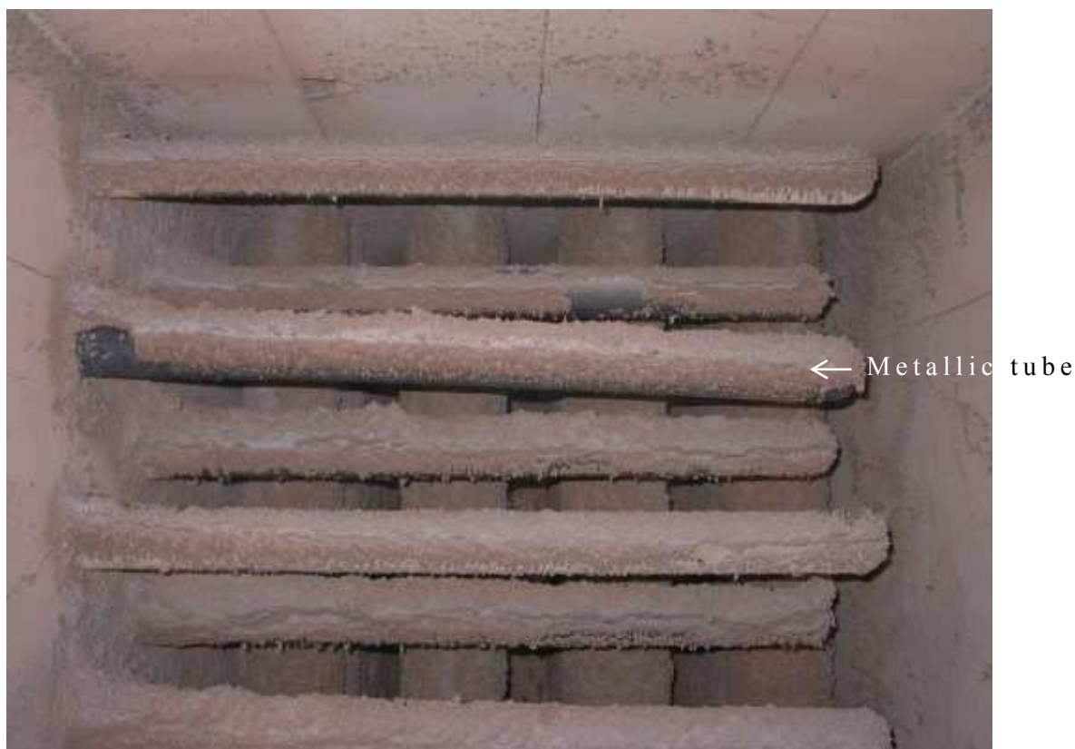
Fig.4.9 SSiC and metallic heat-transfer tubes after exposed 700 hours to exhaust gas.
