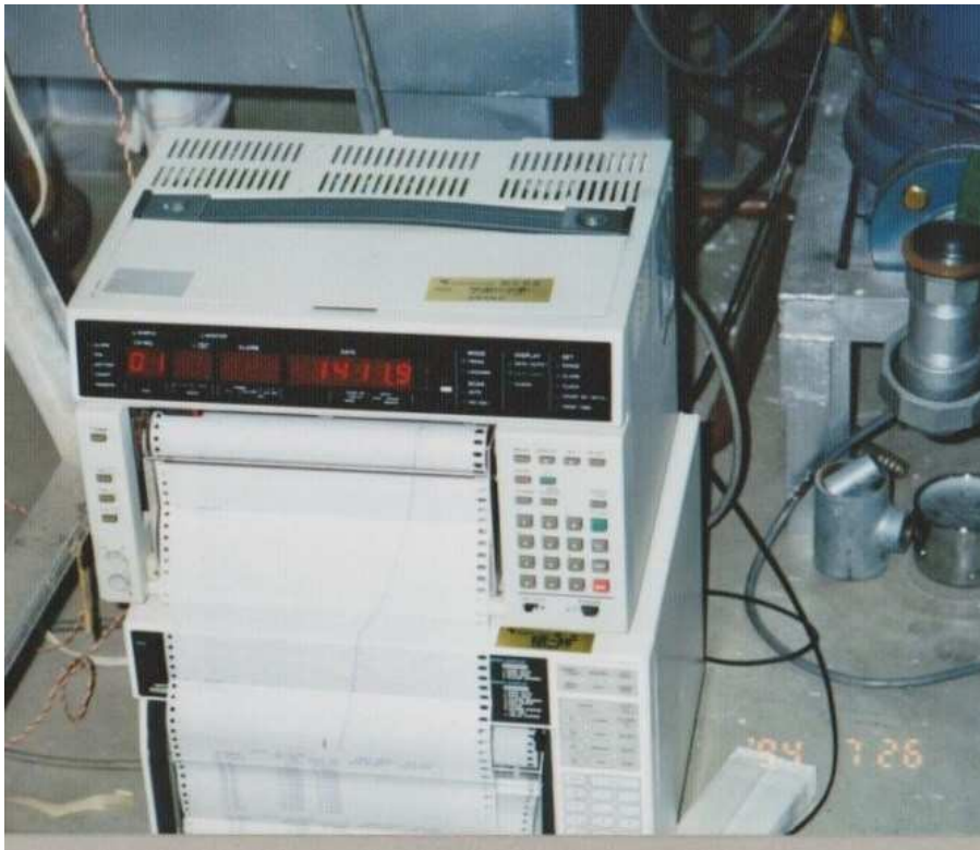
Fig.2.18 Temperature 1670K(1411.9°C) on drawing out test.
