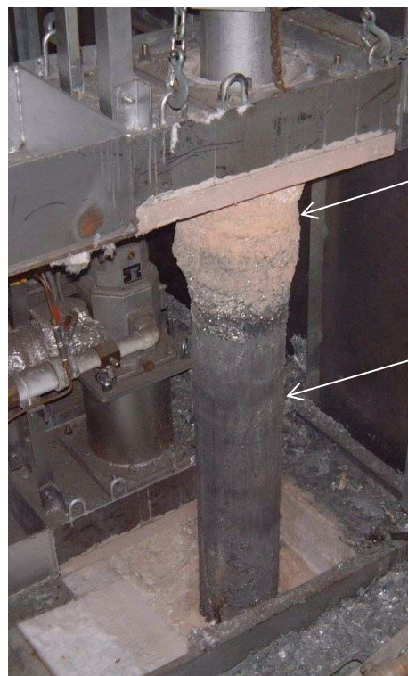
Fig.3.5 View of SSiC immersion tube and dross on galvanizing furnace.
