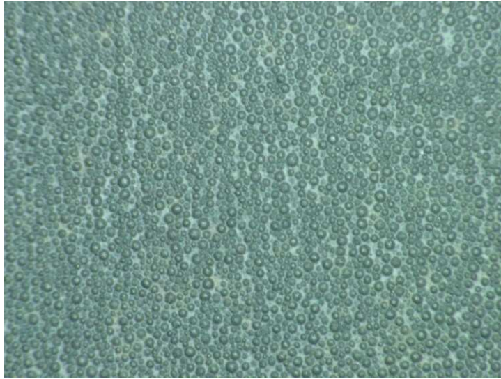
Fig.1.5 SEM image of surface of as sintered SSiC.
