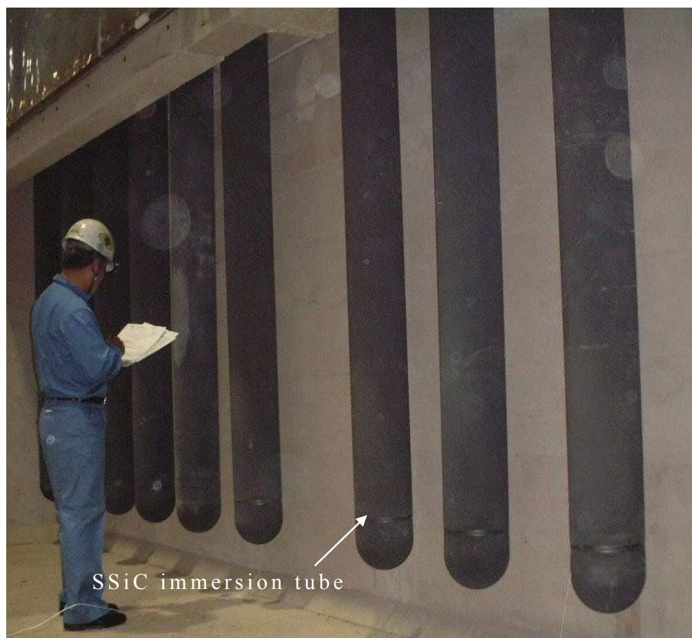
Fig.3.13 View of SSiC immersion tubes in melting bath of zinc.
