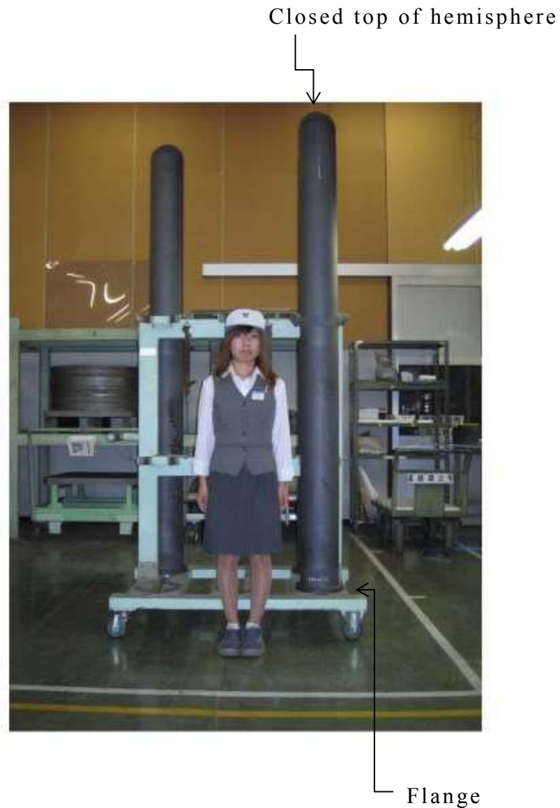
Fig.2.2 Outer tube of SSiC radiant tube of \phi 184 \times \phi 170 \times 2000 mm.
